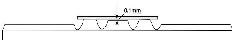
When a cover glass is placed on to these external supports this forms a capillary gap between the rear side of this cover glass and the central support of the counting chamber.
